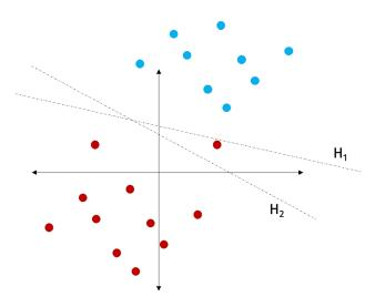
$H_1$  was likely trained with a larger value of C, since its solution has fewer total misclassified points.  $H_1$  more closely approximates the hard margin classifier.  $H_2$  was likely trained with the smaller value of C.
